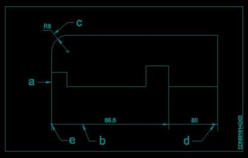
(A) O Dimension line (Correct Alternative) आयाम रेखा (Correct Alternative)
